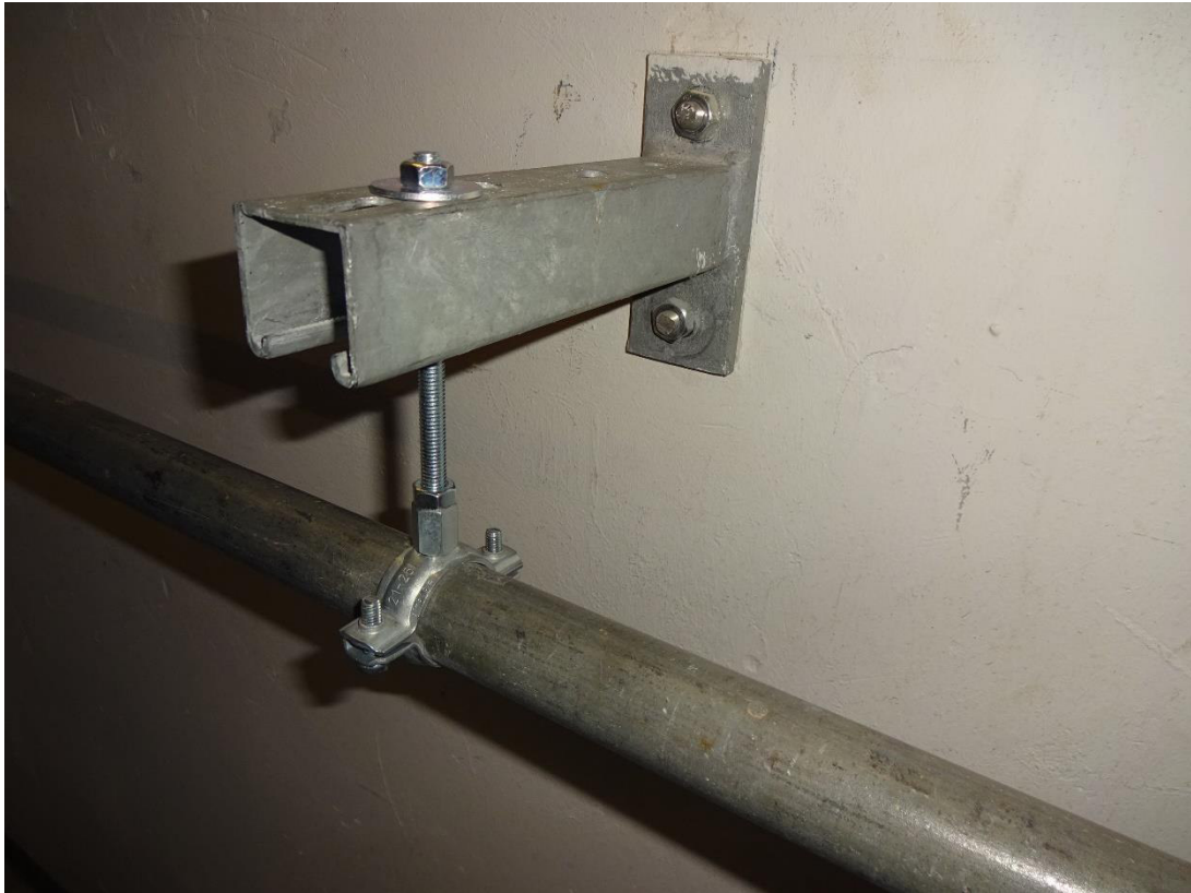
Fig. 1: Reference meas.: DÄMMGULAST®, „Type 1“, rigid fastening without damping element
