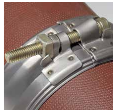
Visual check: After tightening the pipe connector: control slot closed
