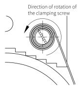
Insert the pointed end of the strap into the slotted screw, then turn the head anti-clockwise. The steel strap wraps around the clamping screw and the strap clamp is tightened.
