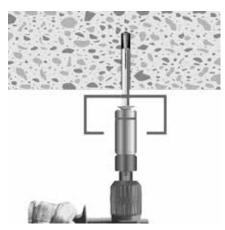
Drive in the MPC-Mounting anchor.
