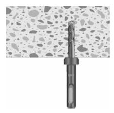
Drill with the MPC-Headed drill.
