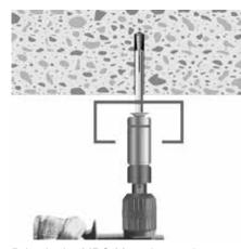
Drive in the MPC-Mounting anchor.
