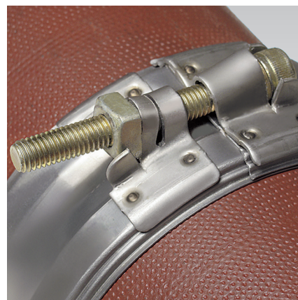
Visual check: After tightening the pipe connector: control slot closed
