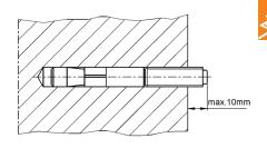
Attachment to building structure: The projecting end of plug or threaded pin from the wall or ceiling must not exceed 10 mm!
