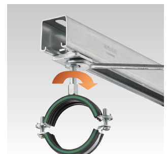
Screw the threaded pin into the MPR-Quick fastener and lock in place with a hexagonal nut. Then mount the pipe clamp
